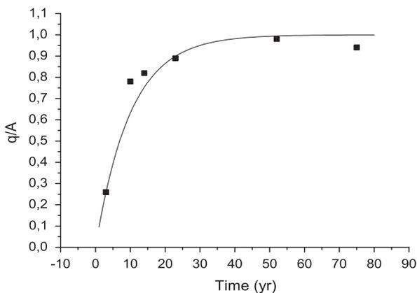
Fig. 1. Normalized yearly flux of sediment at the output of the Quarto Nuovo water reservoir. The squares are the data and the solid line is the fit.
