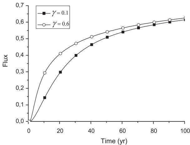
Fig. 3. Normalized yearly flux of sediment at  $x = 2.7$  km for  $\gamma = 0.1/\text{yr}$  and  $\gamma = 0.6/\text{yr}$ ,  $\nu = 0.3$  and  $d = 10^4 \text{ m}^2 \text{ yr}^{\nu-1}$ .
