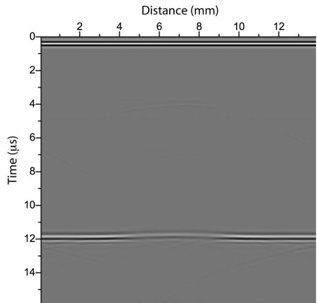
Fig. 6. Time history recorded at the transducer. The reflection event at 12  $\mu\text{s}$  has a smaller travel time and lower amplitude at the location of the tumor.
