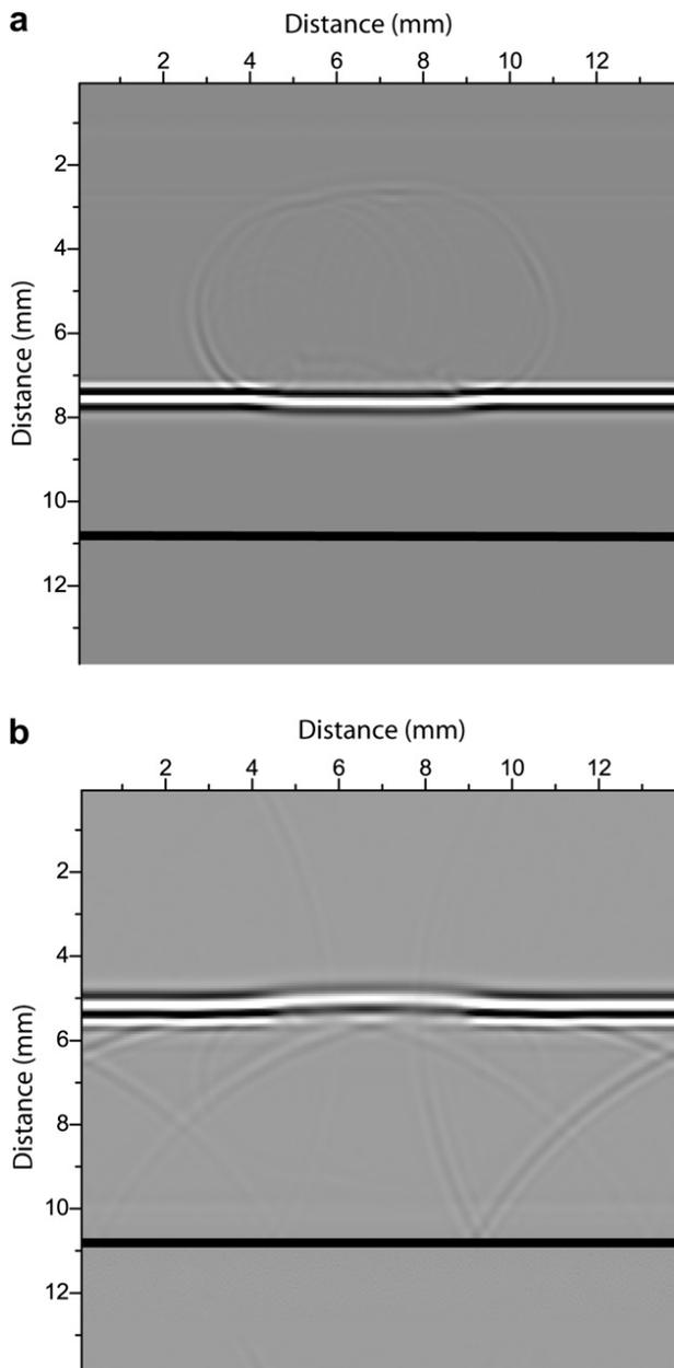
Fig. 5. Snapshots at 4  $\mu\text{s}$  (a) and 10  $\mu\text{s}$  (b). The thick line represents the breast/steel interface and the transducer is located at 2.4 mm (vertical distance). A diffraction event arising from the tumor can be seen at 4  $\mu\text{s}$ .
