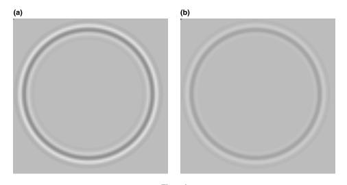
Figure 3 Snapshots of the dilatation field in a lossless medium equivalent to Pierre shale (a), and in a dissipative model of Pierre shale (b).
