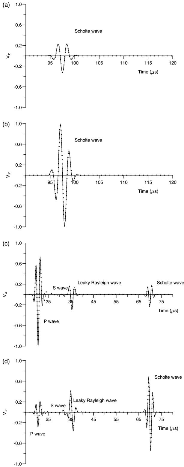
Figure 10. Numerical and analytical solutions (dots and solid line, respectively) of the  $v_x$ -component (a and c) and  $v_z$ -component (b and d), corresponding to the water-Plexiglas interface (a and b) and water-glass interface (c and d). The source is a compressional wave applied to the solid at  $38.4 \mu\text{m}$  from the interface. The receiver is located at the same position and at  $100 \text{ mm}$  from the source. The different waves are indicated.
