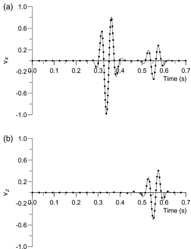
Figure 4. Numerical and analytical solutions (dots and solid line, respectively) of the  $v_x$ -component (a) and  $v_z$ -component (b) corresponding to the water-stainless steel interface. The first event is the direct wave and the second event is the reflected wave.
