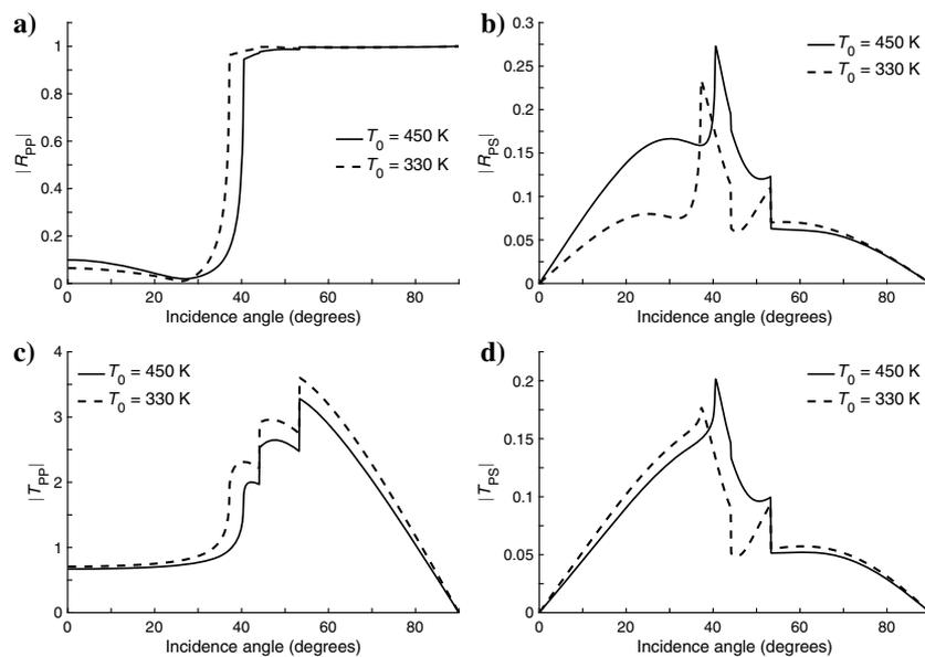
Figure 12. The coefficients of the (a) reflected P-, (b) reflected S-, (c) transmitted P- and (d) transmitted S-waves versus incidence angle  $\theta$  for an incident P-wave at 10 Hz, where the medium properties of  $T_0 = 330$  K correspond to the last column in Table 1 ( $n = 4'$ ). The  $n$  is defined in Figure 1a, and the medium properties are defined in Table 1.
