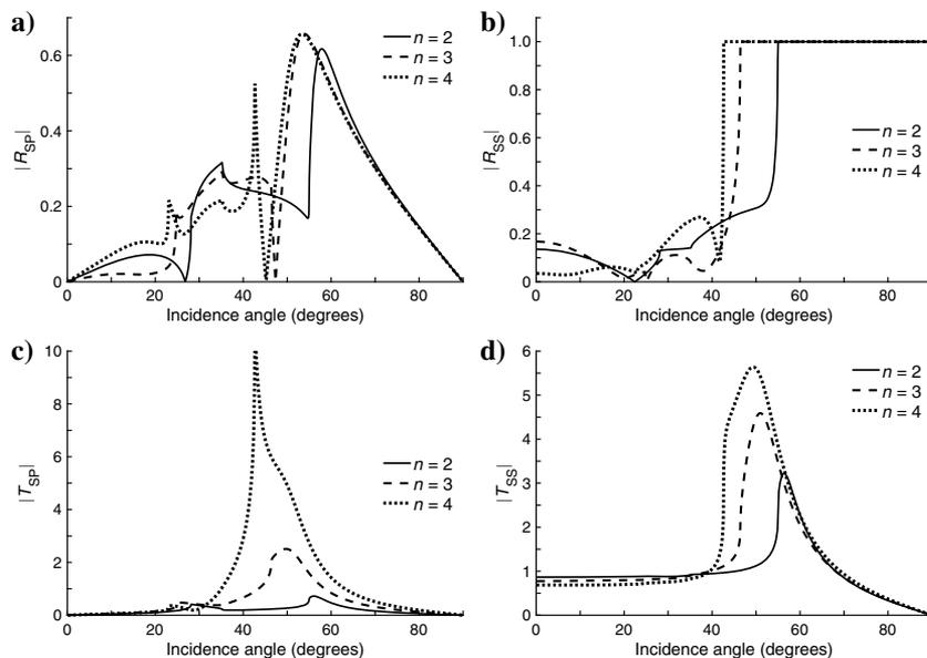
Figure 10. The coefficients of the (a) reflected P-, (b) reflected S-, (c) transmitted P- and (d) transmitted S-waves for the elastic models and an incident S-wave.
