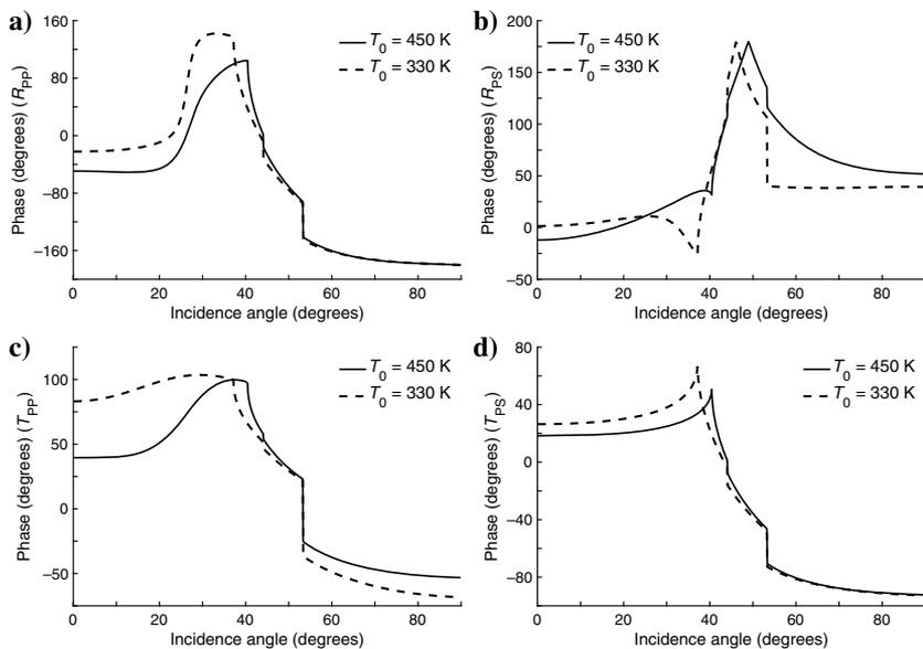
Figure 14. The coefficients of the (a) reflected P-, (b) reflected S-, (c) transmitted P- and (d) transmitted S-waves versus incidence angle  $\theta$  for an incident P-wave, where the frequency is variable and  $n = 4$  is defined in Table 1.
