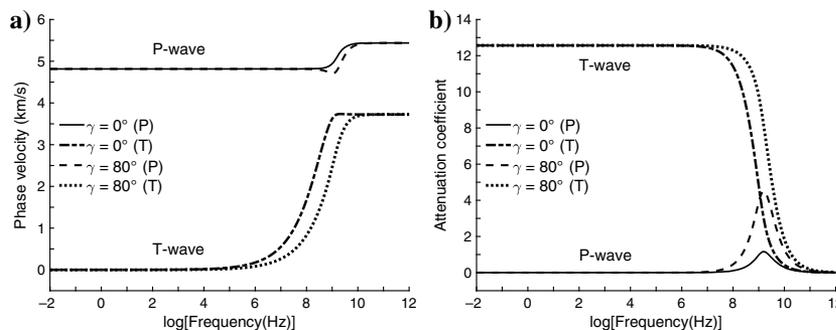
**Figure 2.** (a) Phase velocity and (b) attenuation coefficient as a function of frequency for two values of the inhomogeneity angle  $\gamma$ , where the medium properties correspond to  $n = 4$  in [Table 1](#).
