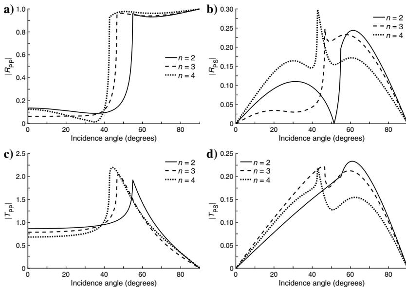
Figure 5. The coefficients of the (a) reflected P-, (b) reflected S-, (c) transmitted P- and (d) transmitted S-waves for the elastic models and an incident P-wave.
