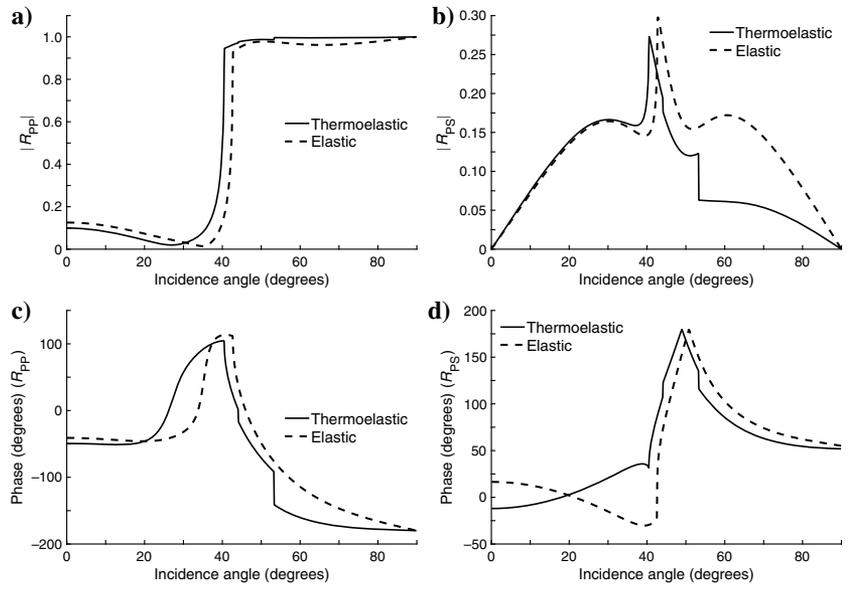
Figure 8. The coefficients of the (a) reflected P-, (b) reflected S-, (c) transmitted P- and (d) transmitted S-waves versus incidence angle  $\theta$  for an incident S-wave at 10 Hz. The  $n$  is defined in Figure 1a and the medium properties are defined in Table 1.
