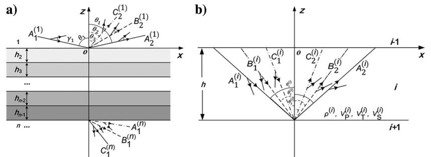
Figure 1. (a) R/T of waves in a multilayered medium and (b) details of the  $i$ th layer. The solid, dotted solid, and dashed lines represent the propagation direction of the incident P-, T-, and S-waves, respectively.
