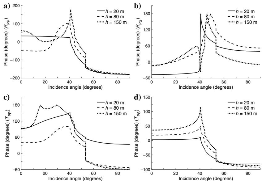
and layer thicknesses of the cap rocks. The coefficients of the reflected and transmitted P-waves for different temperatures are similar, whereas the amplitudes of the S-waves are higher for higher temperatures. The reflection coefficients can be used to obtain information about the thermal characteristics of a multilayered medium, which provides theoretical support for HDR geothermal exploration.
