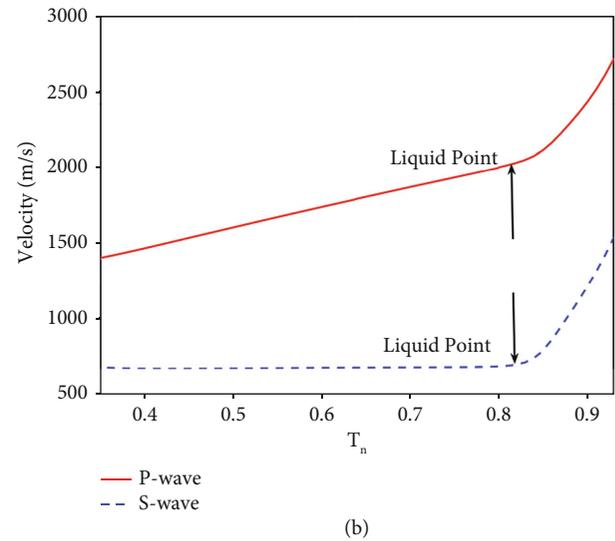
FIGURE 15: P- and S-wave velocities of the heavy oil sand (sample #9 at 1100 psi effective pressure) as a function of temperature (a) and normalized temperature (b).
